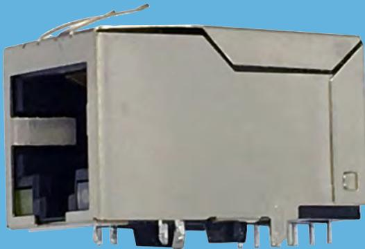
The RJ45 jack with shortened contacts for pin-in-paste technology makes it possible to use efficient manufacturing processes. This allows pick & place robots Tape & Reel packaged SMT (Surface Mount Technology) and PiP components to be installed in the same process and IR reflow soldering.
